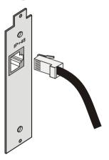
Figure 2-6: LAN IP network connection
